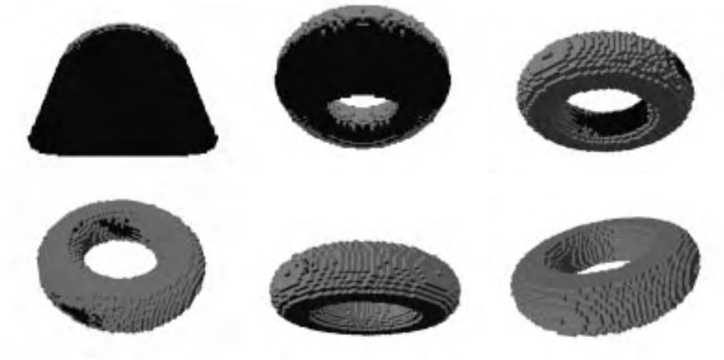
Figure 19: The Optimal Method volumetric models after the acquisition of each view (from left to right and top to bottom). Each model is oriented in the direction of the view to be acquired next.
