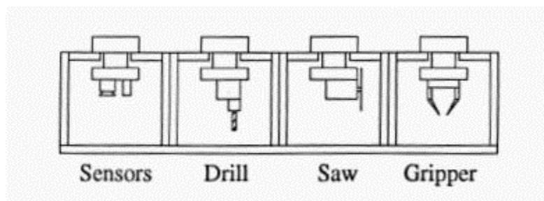
Figure 4. Interchangeable modules from the toolrack for dismantlement
