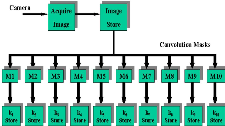
Figure 8. Block diagram of the real-time implementation of the facet model
