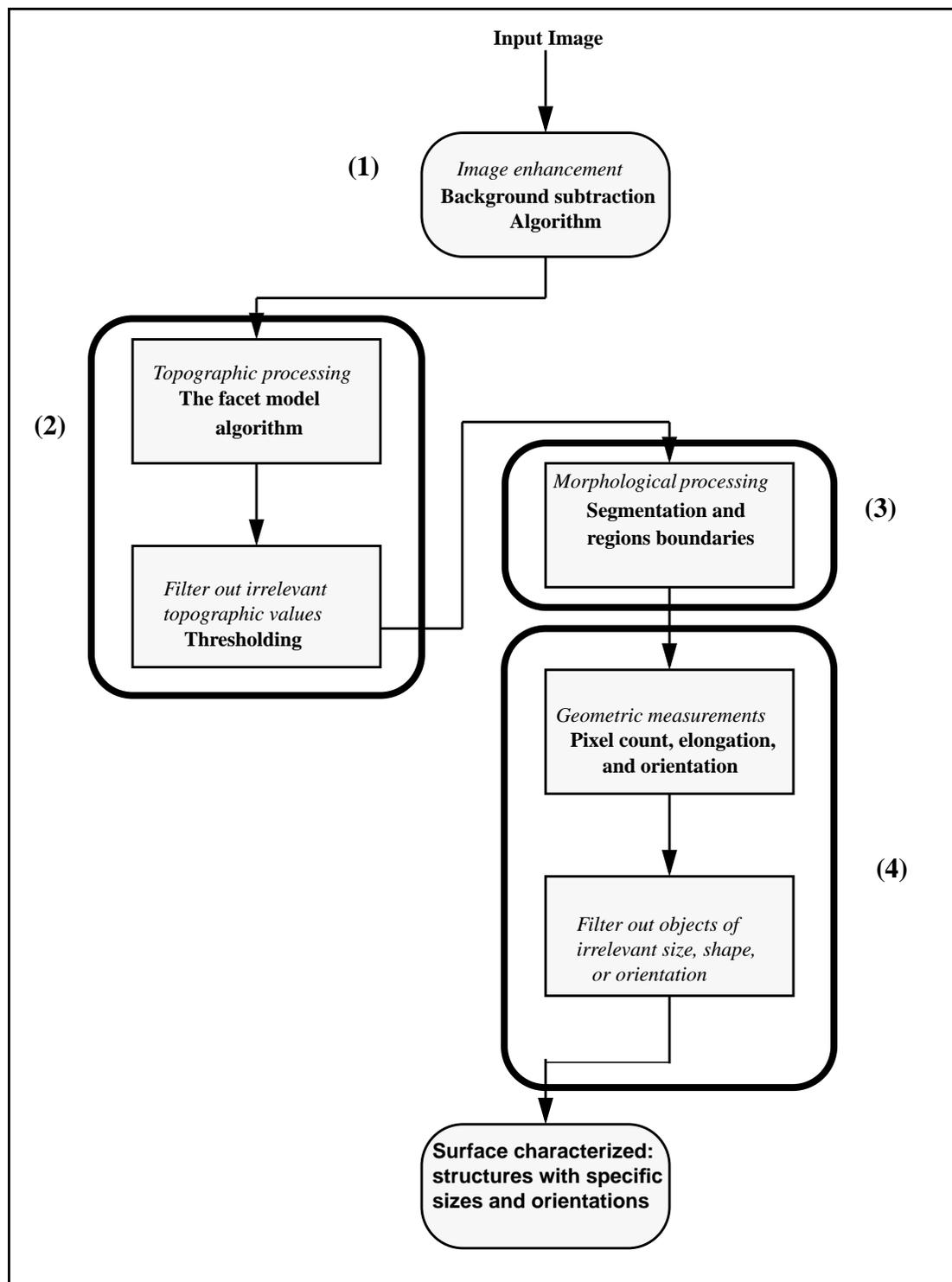
Figure 1. Block diagram of the surface characterization algorithm
