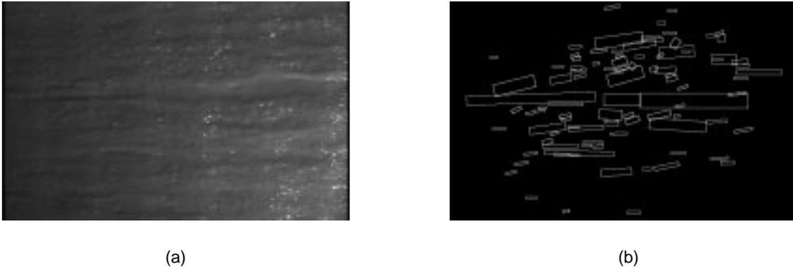
Figure 7. (a) Original image of the slurry, (b) results of the surface characterization algorithm(MBR).
